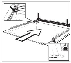
■ Push the middle pane (where present) into the frame almost to the end. The material (M-) number printed on the pane must be legible in the bottom right hand corner (see illustration). Fit the sealing strip into position, then push the pane in as far as it will go.
